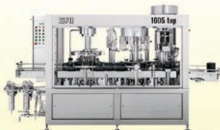
BOTTLING MONOBLOCKS WITH RINSING, DE-AERATION & GASSING, FILLING SCREW CAPPING (STELVIN OR STELVIN LUX) OR CORKING (OR BOTH), AVAILABLE AS INDIVIDUAL MACHINES. PRODUCTION RATE FROM 1000 BPH
